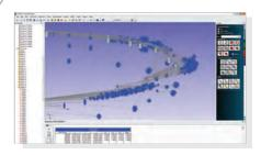
A powerful feature that leverages the uncertainty characteristics of different instruments to provide a much more accurate instrument network than that of traditional alignment methods.
