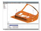
A variety of alignment methods ranging from traditional 3-2-1 alignments to more advanced surface fits.
